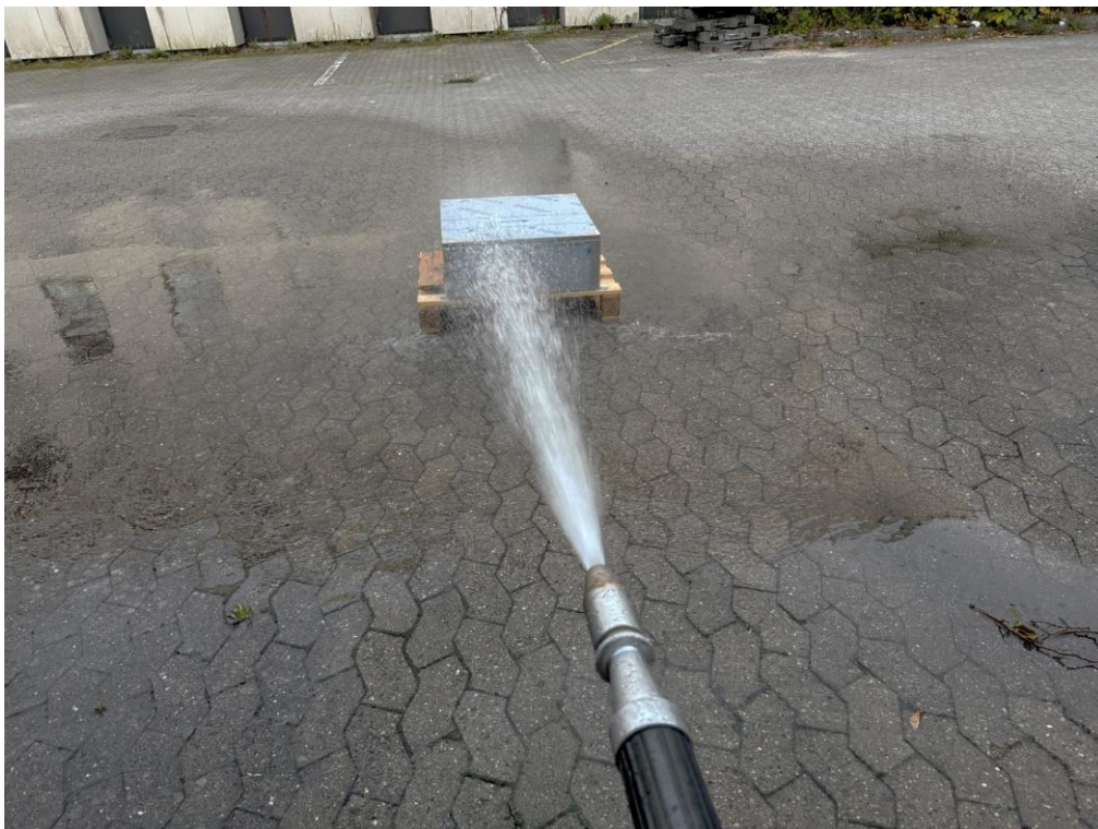
Photo 11 During exposure, IPX6. Side 2.
