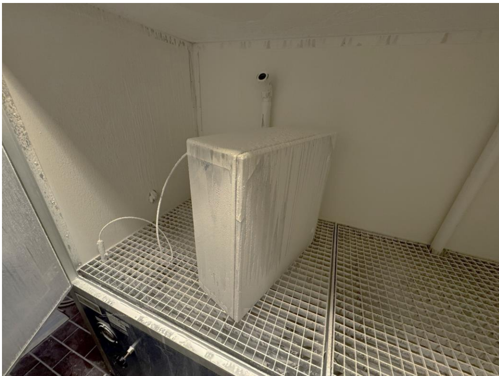
Photo 3 After exposure, IP6X.
