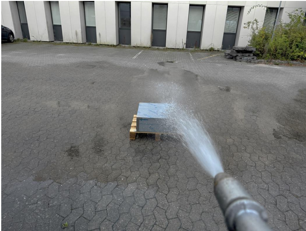
Photo 14 During exposure, IPX6. Top.
