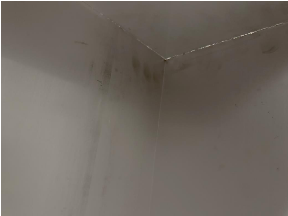
Photo 6 Visual inspection, IP6X. No ingress of dust observed.
