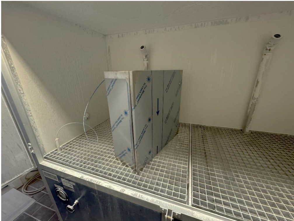
Photo 2 Before exposure, IP6X.
