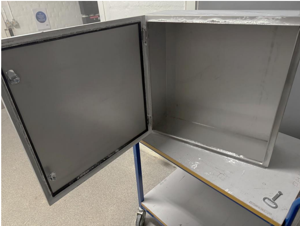
Photo 4 Visual inspection, IP6X. No ingress of dust observed.
