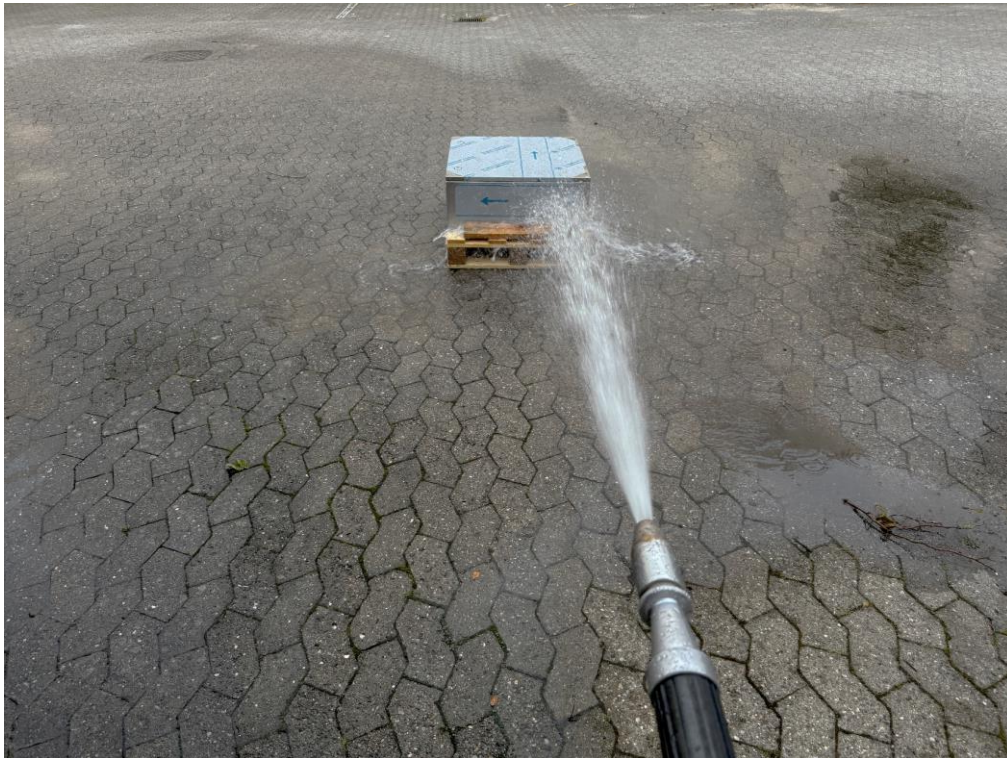
Photo 10 During exposure, IPX6. Side 1.
