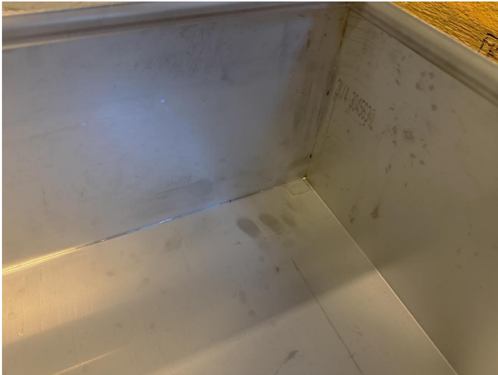
Photo 16 Visual inspection, IPX6. No ingress of water observed.
