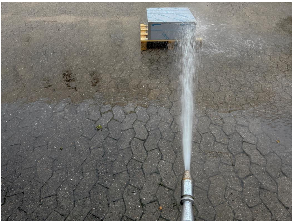
Photo 13 During exposure, IPX6. Side 4.
