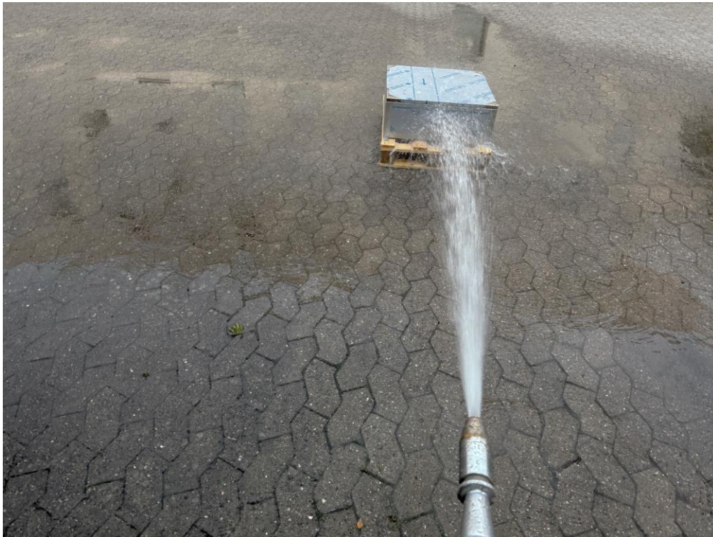
Photo 12 During exposure, IPX6. Side 3.
