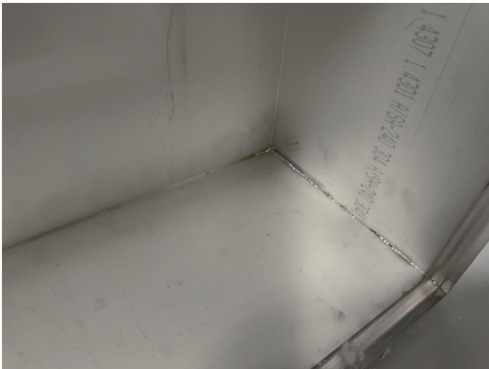
Photo 5 Visual inspection, IP6X. No ingress of dust observed.
