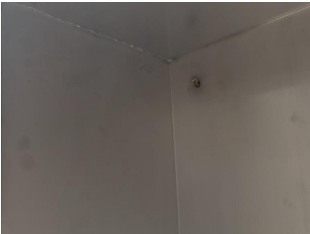
Photo 7 Visual inspection, IP6X. No ingress of dust observed.
